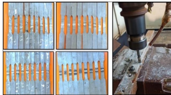
Figure 7. Formed tensile strength specimens
